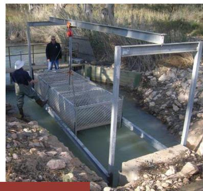
*Both the jumping and pushing traps proved a great success in removing large numbers of carp (around 8 tonne in 4 months) and both show great promise for wider application in fishways and irrigation channels.*
