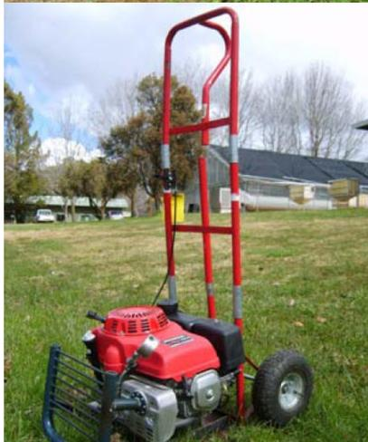
Prototype CO pressure fumigators
