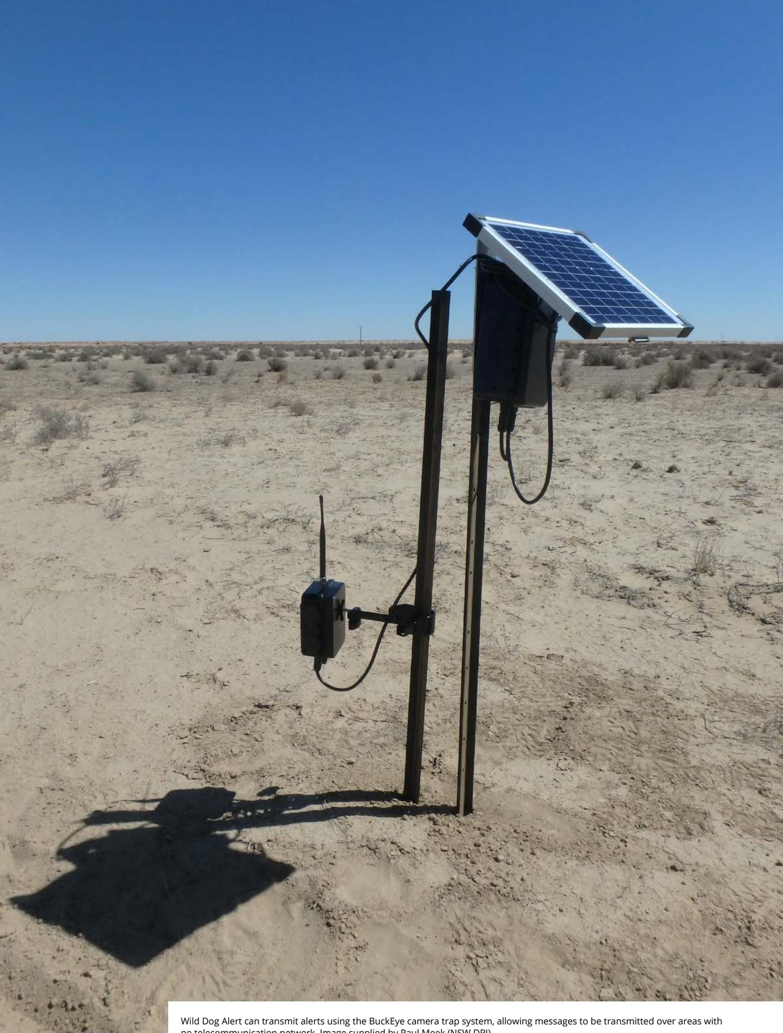
Wild Dog Alert can transmit alerts using the BuckEye camera trap system, allowing messages to be transmitted over areas with no telecommunication network. Image supplied by Paul Meek (NSW DPI).
