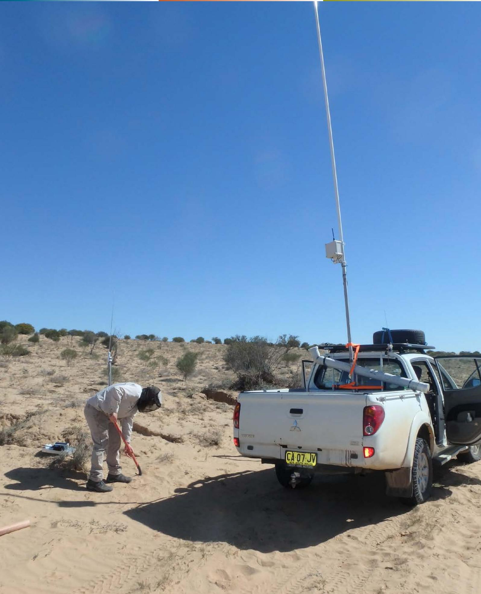
As part of wild dog alert, testing the Celium alert system under harsh Australian conditions was critical to designing the trap alert platform, here Heath Milne is burying a trap alert mole to conduct a drive test to measure transmission distance in the desert. Image by Dr Paul Meek (NSW DPI).
