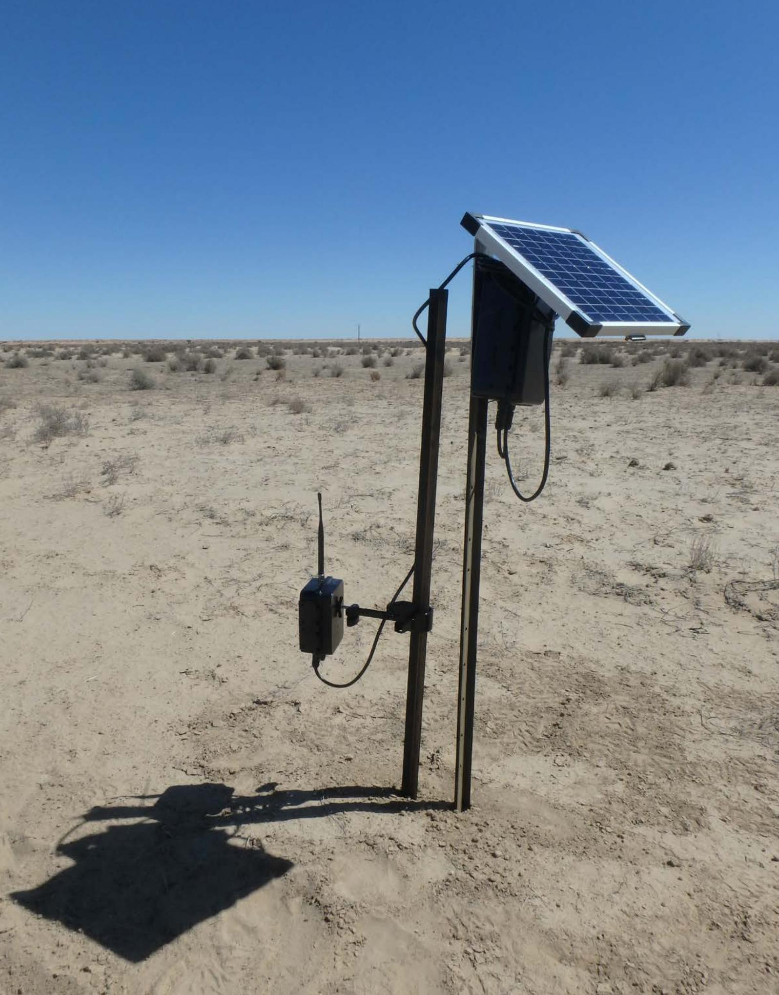
Wild Dog Alert can transmit alerts using the BuckEye camera trap system, allowing messages to be transmitted over areas with no telecommunication network. Image supplied by Paul Meek (NSW DPI).
