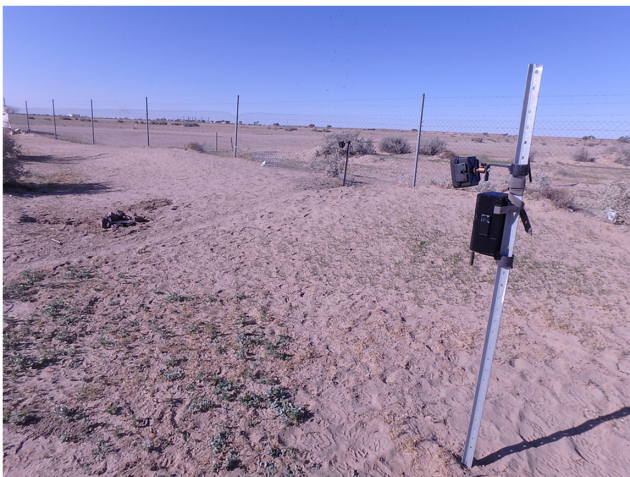
Fig. 4. Field deployment involved positioning of the SBS camera unit at 1 m height and 4–5 m distant from the ground dispenser unit.
