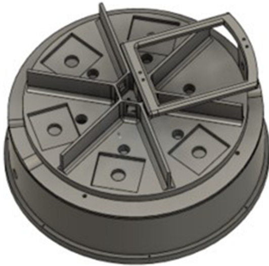
Fig. 3. Computer-aided design (CAD) image of the bait dispenser showing the internal carousel design (the square structures within each triangle segment are the bait chambers and the empty segment is the starting point).
