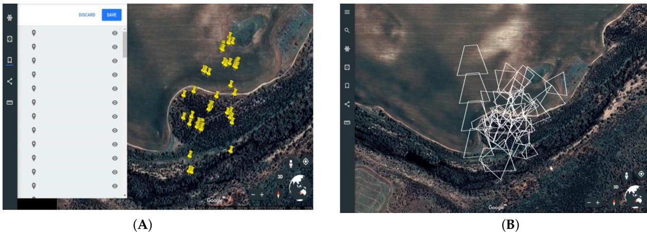
Figure 7. (A) The geo-tagging of detected animals from drone data that points out their detection location and (B) visualisation of animal movements that display the area of their activity.
